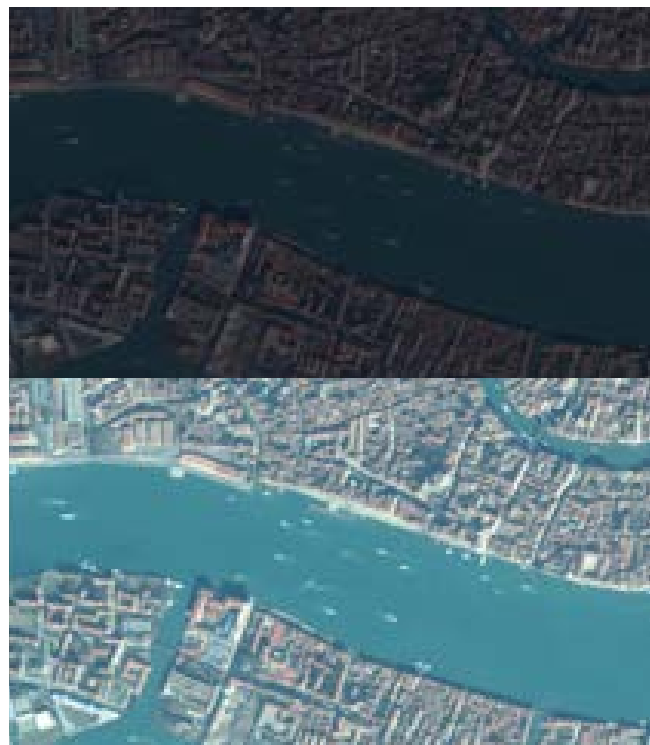
Figure 3.9: Example of an 8-bit product without linear adjustment (top) and with linear adjustment (bottom).
