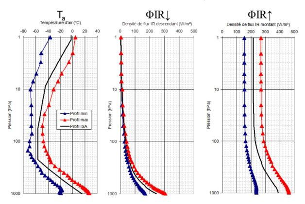
Densities of upward ( $\Phi IR\uparrow$ ) and downward ( $\Phi IR\downarrow$ ) infrared flux in clear sky conditions from CNES model based on temperature (T<sub>a</sub>) profiles
