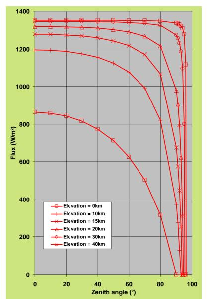
Solar constant and example of direct solar flux density in atmosphere.
