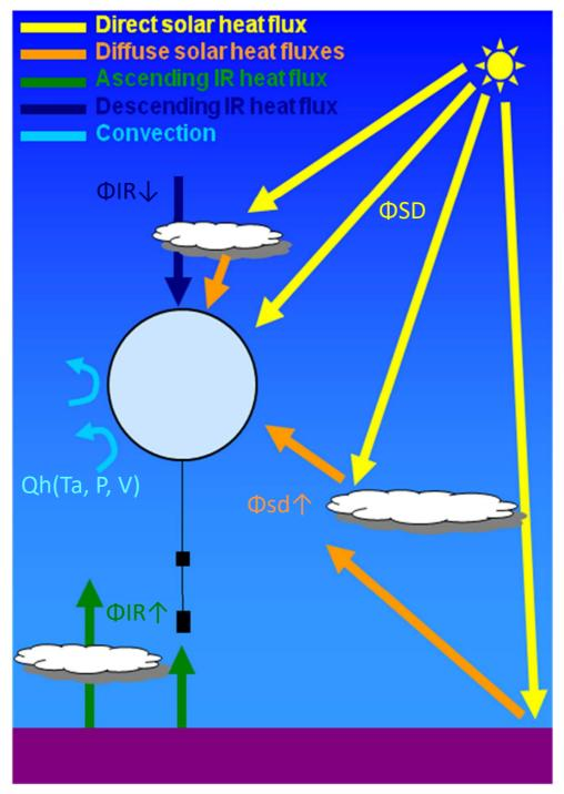
Heat Transfer Modes and Thermal Environment Parameters for Payload Gondolas
