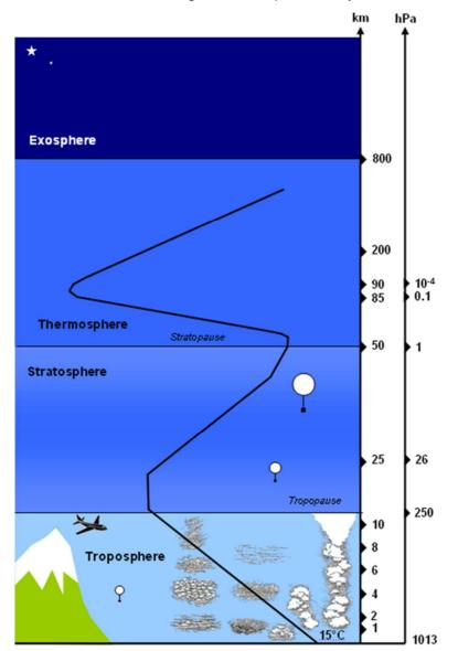
Standard Atmospheric Profile along the Pressure and Altitude Scales
